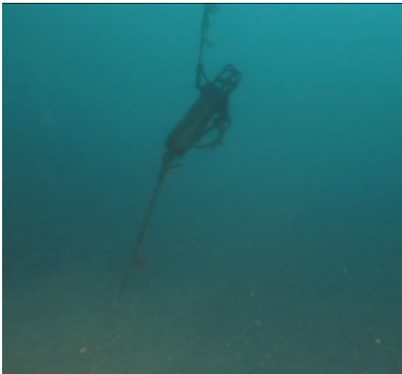
One of our SAMARUC systems deployed in "El Gorguel" for the assessment of ambient noise levels.
