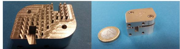
Figure 4. Filter base piece with periodic bed of nails, shortened cylindrical resonant nails, and input-output GGWs
