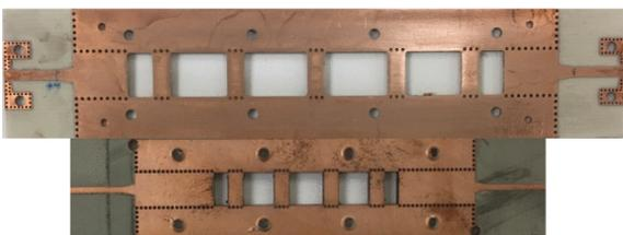
Figure 3. Manufactured filters. 13 GHz and five cavities filter with RO4003C (top) and 11 GHz and four cavities filter with TMM10i (bottom)
