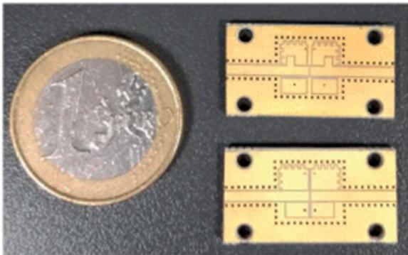
Figure 6. Photograph of filter prototypes: above filter DB2, and below filter DB1
