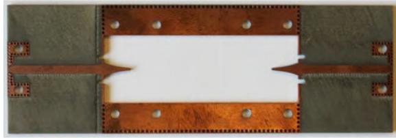
Figure 8. Manufactured prototype of the back to back transition from microstrip to ESIW
