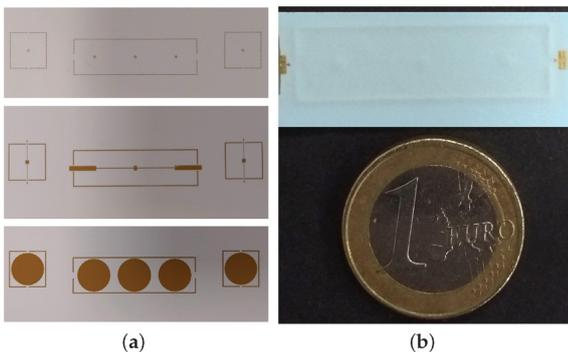
Figure 7. (a) Some layers of the LTCC stack-up and (b) Three-pole BPF prototype
