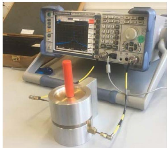
Figure 5. Measurement setup: VNA and split-cylinder resonator
