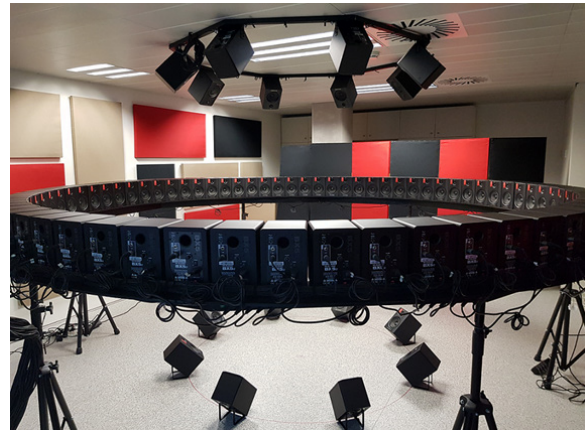
Fig. 1. Perceptual spatial acoustic laboratory including a render system of 72 + 16 loudspeakers.
