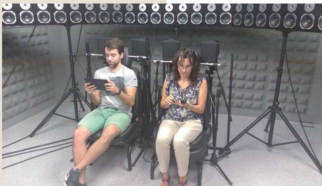
Figure 1. Prototype of sound field control system for two listeners. Location: GTAC listening room.
