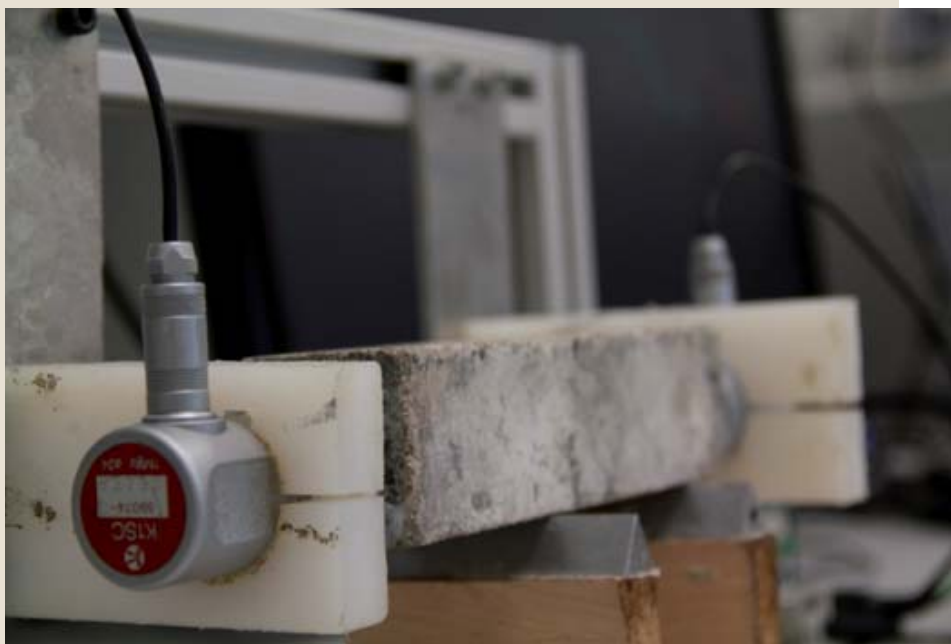
ONDATEST damage characterization by means of US.
