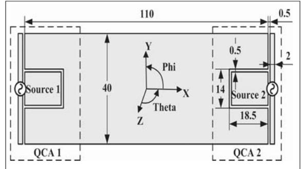
■ **Figure 13.** MIMO prototype antenna with two QCA basic structures at both end of the ground plane. Dimensions are in mm.
