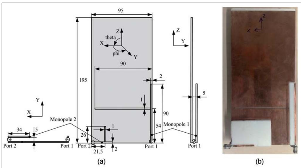
■ **Figure 10.** (a) Planar radiating ground plane with monopoles of two different lengths as coupling elements. The gray color is metal, whereas the white color is air. Dimensions are in mm. (b) Prototype of the antenna.
