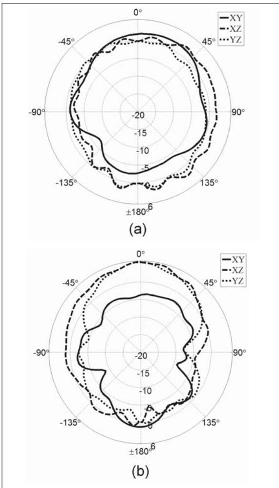
■ **Figure 16.** Measured radiation patterns of QCA 2 at (a) 2 GHz and (b) 5 GHz in terms of total gain (dBi).
