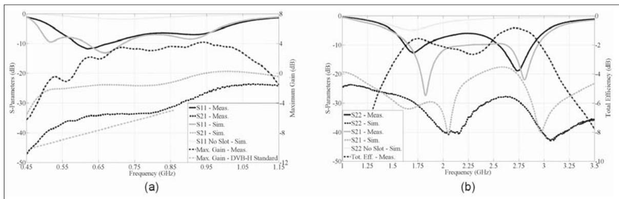
■ **Figure 11.** Measured and simulated S-parameters (a) for Monopole 1, with measured maximum gain and (b) for Monopole 2, with measured total efficiency. Simulated S-parameters are compared with the case without slot.
