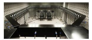
Fig. 1. Acoustic listening room including a render system of 96 loudspeakers.
