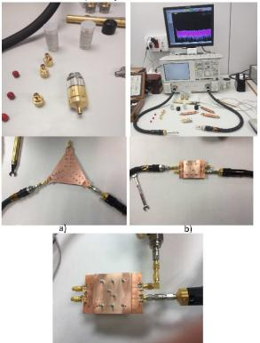
Figure 7. Measurement of the frequency response of the devices. Calibration kit and measurement setup. Detail of the measurement process.
