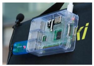
Fig. 4. Node formed by a Raspberry Pi, one microphone and one solar panel.
