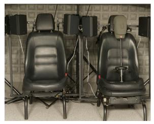
Fig. 3. Laboratory prototype of a system implementing multiple personal sound zones with two real car seats.
