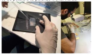
Figure 4. Filling of a glass cell and a microwave device with liquid crystal
