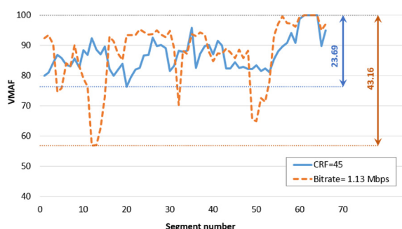
Comparison of the VMAF value of each segment of the "Elephants Dream" video encoded at constant quality (CRF 45) and constant bitrate (1.13 Mbps)
