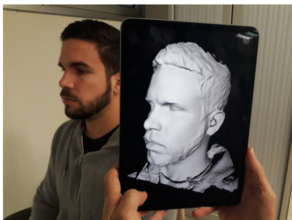
Figure 5. Creation of a 3D model for HRTF characterization.
