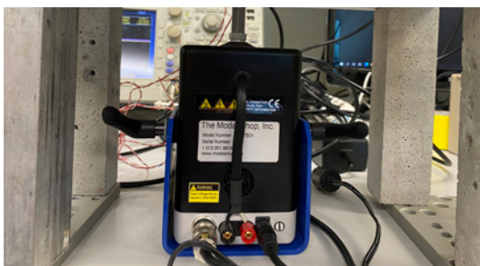
Automatic impact hammer system.
