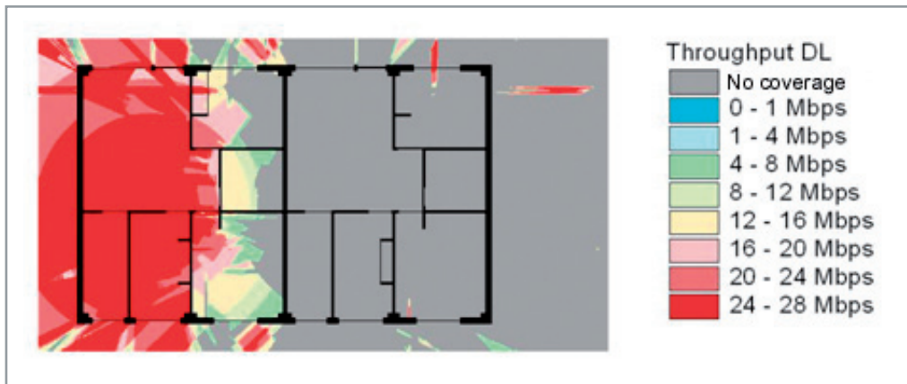
■ Figure 4. Left flat throughput, two femtonodes located in central locations in neighbour homes
