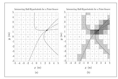
**Figure 2**. Intersecting half-hyperboloids and localization approaches. (a) Conventional SRP-PHAT. (b) Proposed.
