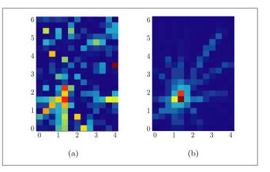
**Figure 4**. Source likelihood map when a coarse grid is used. (a) Traditional and (b) modified SRP-PHAT.
