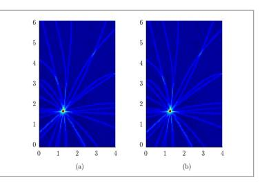
**Figure 3**. Source likelihood map when a fine grid is used. (a) Traditional and (b) modified SRP-PHAT.
