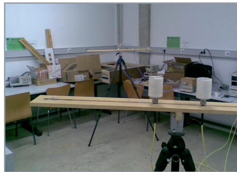
■ Figure 15. Two omnidirectional UWB antennas EM-6116, with 1dBi gain.
